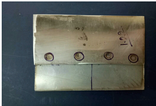
Fig 7. Workpiece after Spot Welding of Thickness
