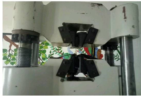
Fig. 8. Tensile stress check of the workpiece
